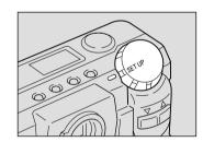
Press the button to select or [FORMAT] and press the ENTER button.
